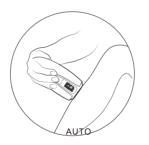
❖ Press o and o hold for 2seconds to switch mode between "Auto" and "Manual"
